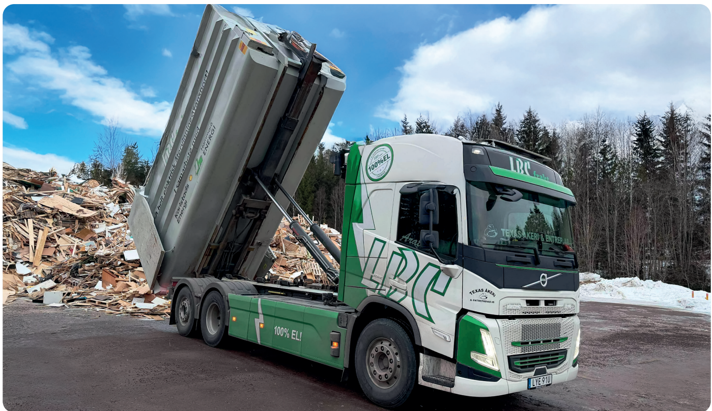
One of Texas Åkeri & Entreprenad's Volvo FM Electric 6x2 R trucks unloading construction waste at a local recycling centre, fitted with a MULTILIFT ULTIMA 20ZL 53 hooklift.
